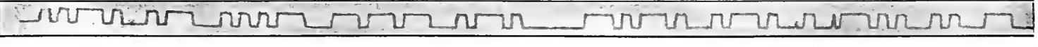
HOW SHORT WAVE HIGH POWER— A section of tape, part of a message received at the Broad Street offices of the Radio Corporation of America from station SAQ at Gothenburg, Sweden. The message reads: "Favor creditbank Oslo 2." The effects of static can be seen in several places appearing as a sharp pointed mark much narrower
